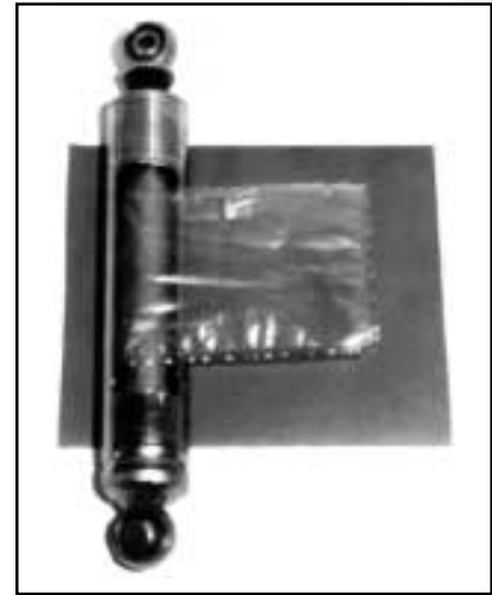
Other manufacturers' "gas cell" bag. These bags fail prematurely, causing shock fade.
